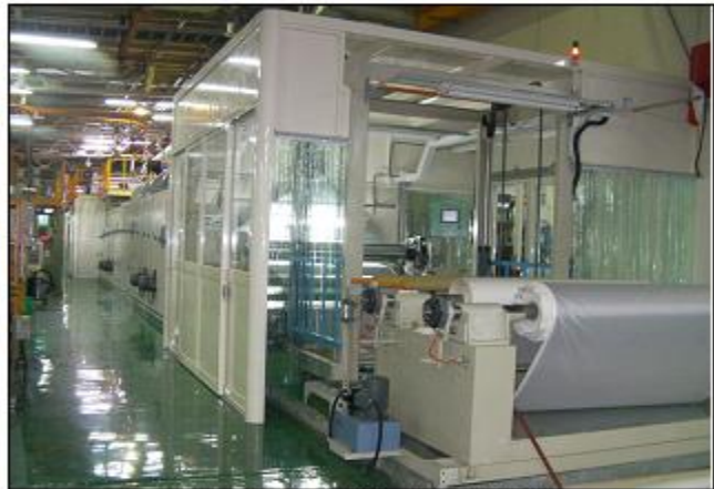
離型紙複合材料製膜機整廠設備 Composite Film Processing Plant
